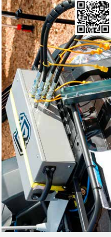
HYDRAULIC POWER UNIT
